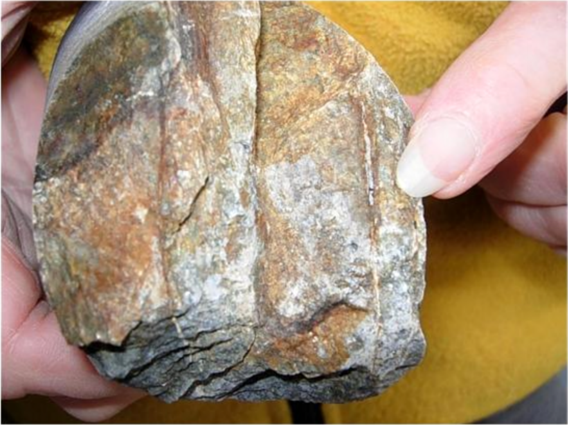
Figure 5.10.3-3(a). Vertically oriented calcite-filled vein with sulfide minerals (tentatively identified as pyrite and arsenopyrite). Depth interval = 108.25-108.4 ft.
