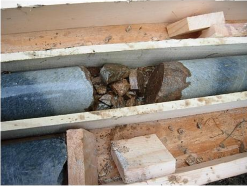
Figure 5.10.3-1. Large open fracture at approximately 39 ft. bgs. Note wide bands (several cm thick) of iron oxidation adjacent to fracture surface.
