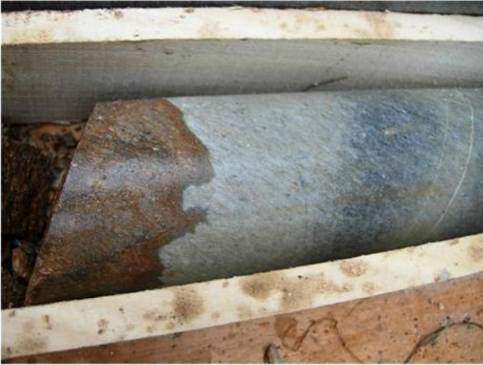
Figure 5.10.3-2. Close-up of fracture in Figure 5.10.3-1 showing bleached zone surrounding iron-oxidation band; bleaching is inferred to be relict hydrothermal alteration.
