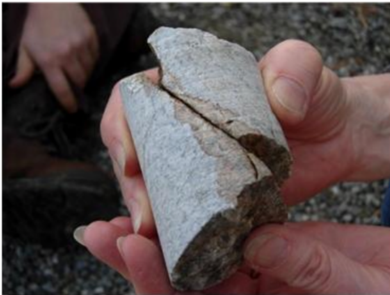
Figure 6.1.2-1. Core from N5 showing alteration (Fe oxidation) along a fracture surface.
