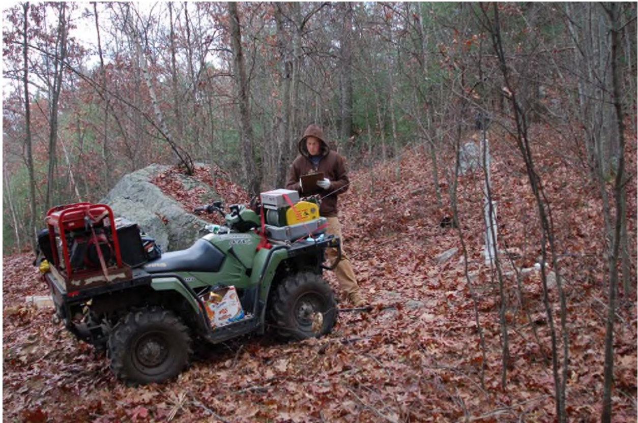
Figure 1 – Borehole logging setup using HGI's all-terrain vehicle (quad)
