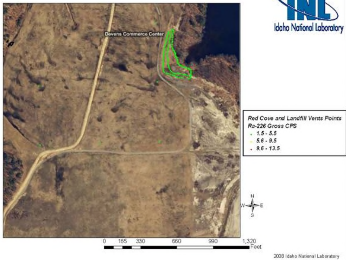
Figure 8c. Ra-226 gross count rate data collected at Red Cove and vents on the Deven's landfill cover.
