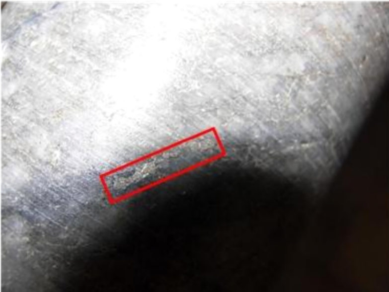
Figure 5.10.3-3(b). Quartz vein with silver-colored sulfide mineral (possibly arsenopyrite). Depth interval ~133 ft.
