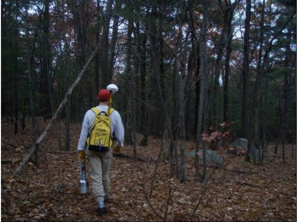
Figure 2. BaSIS system and operator conducting NORM radiation survey at Shepley's Hill site. Note: The radiation detector is to the left of operator.
