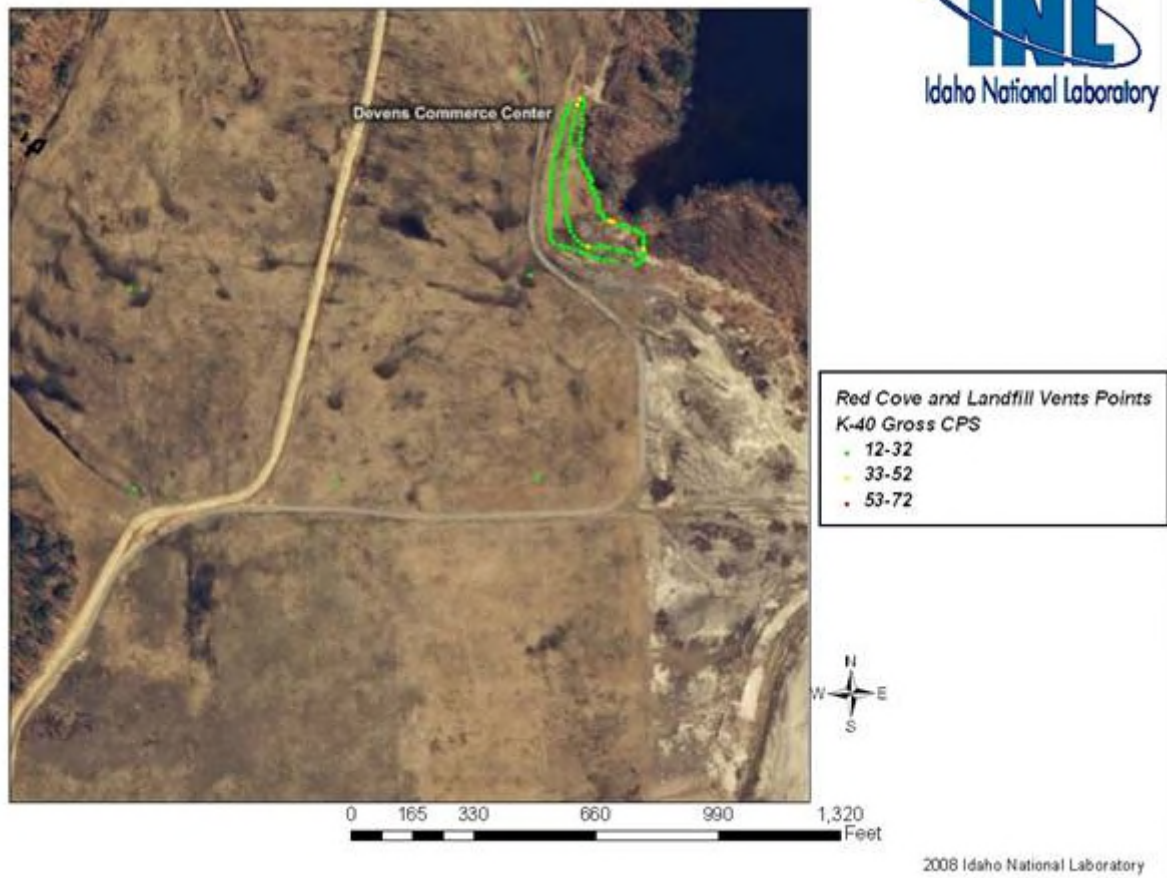
Figure 8b. K-40 gross count rate data collected at Red Cove and vents on the Deven's landfill cover.
